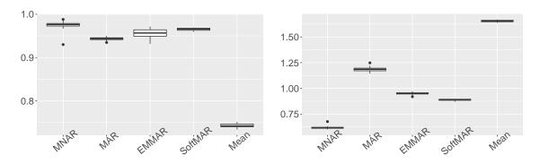
Figure C.9: RV coefficients for the loading matrix (left) and imputation error (right) when r = 2, n = 1000, p = 50 and twenty variables are MNAR.
