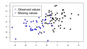
Figure 2.1: Introduction of MNAR missing values using a logistic regression (2.14), with  $\phi_1 = 3$  and  $\phi_2 = 0$ . One can see that the highest values of  $y_{i1}$  are missing, mimicking a cutoff effect.
